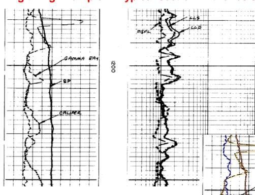
To left: Typical scanned image of resistivity log showing, GR, SP, CALI, LLD, LLS, and MSFL traces shown in greyscale. Digitising these lines can be difficult using traditional digitising techniques.
